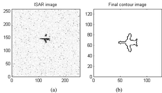
Fig. 9. ISAR image received (a) and optimized (b).
