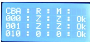
Fig. 19. Result of the testing of the tri-state output network (with the network on Fig. 6)
