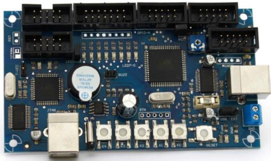
Fig. 12. AVR development board „T-Bird 2”
