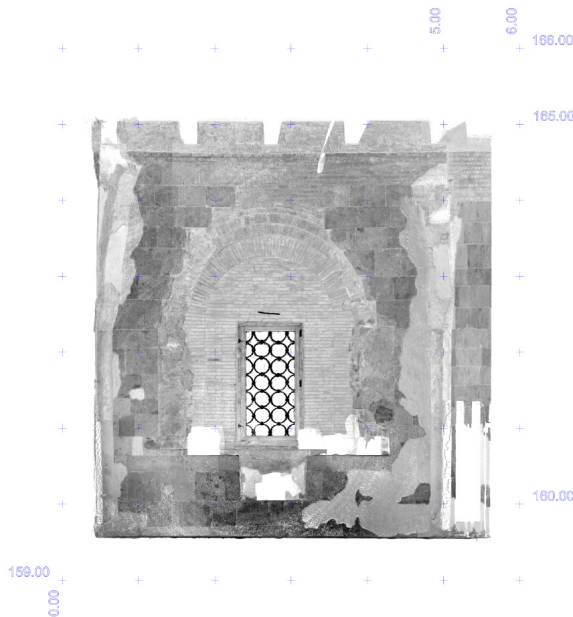
Figure 3. Intensity colored orthoview of a wall with the overlay grid and labels (left) and detail from panorama picture about the same wall made by laser scanner (right)
