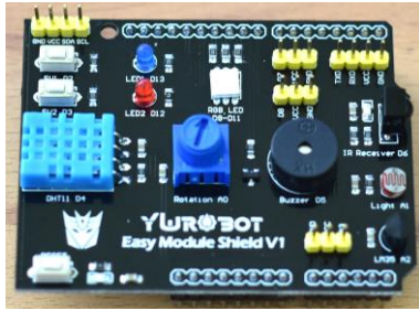
Figure 4. The YURobot Easy Module Shield v1
