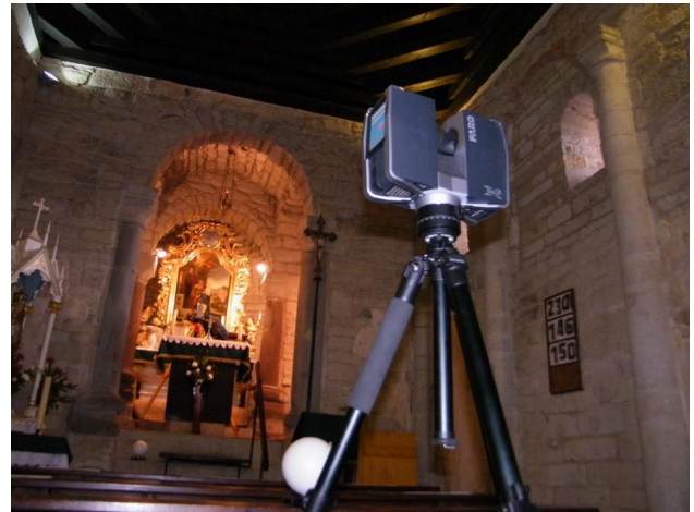
Figure 4. Surveying using a laserscanner
