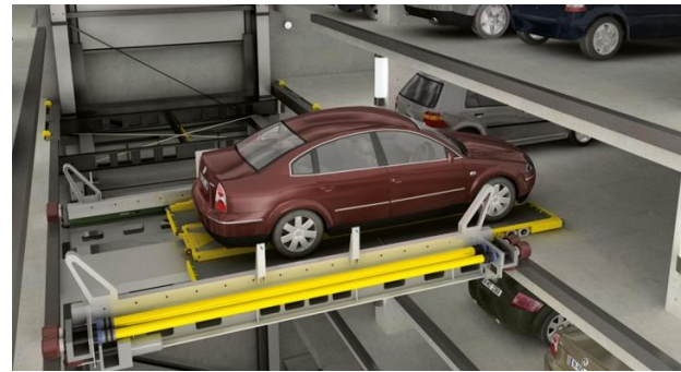
Figure 7. Loading cars by tire-grabber in robotic parking system (without applying car storage pallet) [5]
