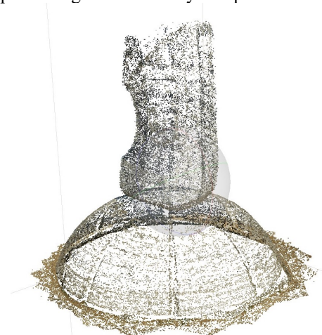
Figure 3. The point cloud model generated by automatic image matching procedure (PhotoScan)
