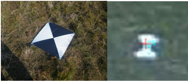
Figure 2. Ground control point sign and its image
