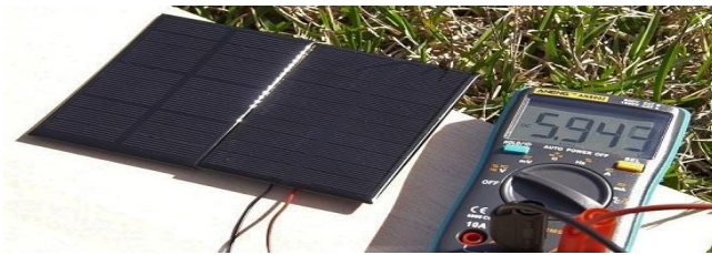
Figure-6. Measurement of solar panels with a multimeter
