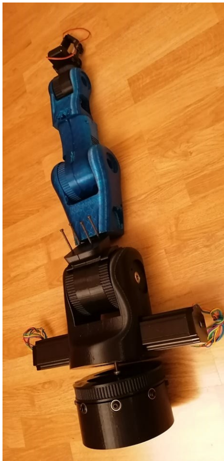
Fig. 2: Assembly of BCN3D Moveo
