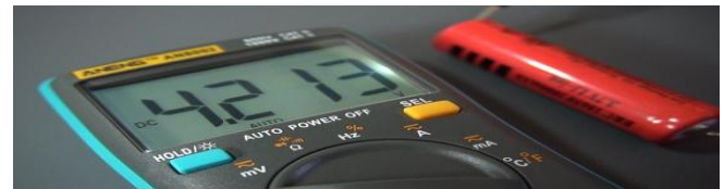
Figure-10. Measurement of lithium batteries with a multimeter
