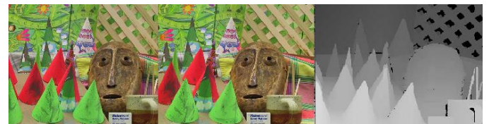
Figure 4. Applying SGM on a pair of images (source: http://lunokhod.org )
