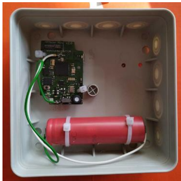
Figure 1. Sensor unit with 3 axes accelerometer
