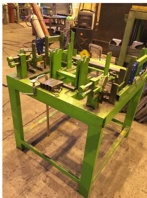
Fig. 10.: Individually designed welding jig
