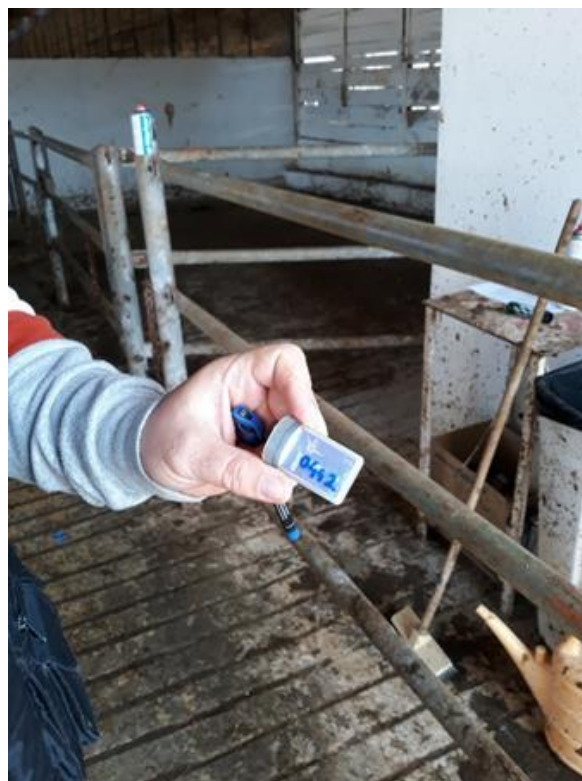
Figure 4 Lying data logger with the cattle ID
