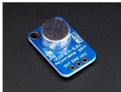
Fig. 8. MAX4466-based electret microphone with adjustable gain
