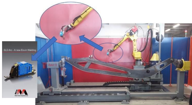
Fig. 1: Robot welding with sensor
