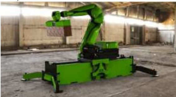
5. Figure KM Robotics mobile brick laying robot application []
