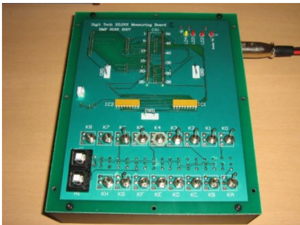
Figure 7. XILINX CPLD Programmable Logic Integrated Circuit (PIC) based test box (own editing)
