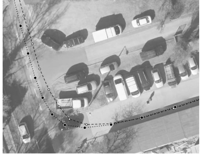
Fig. 3. Ortophoto of the experiment site, with the trajectory of measured GPS (white circles, dashed line) and the Kalman filter processed coordinates (black dots, dotted line). This site is the first turn, where the processed trajectory properly fits on the edge of the bike lane.
