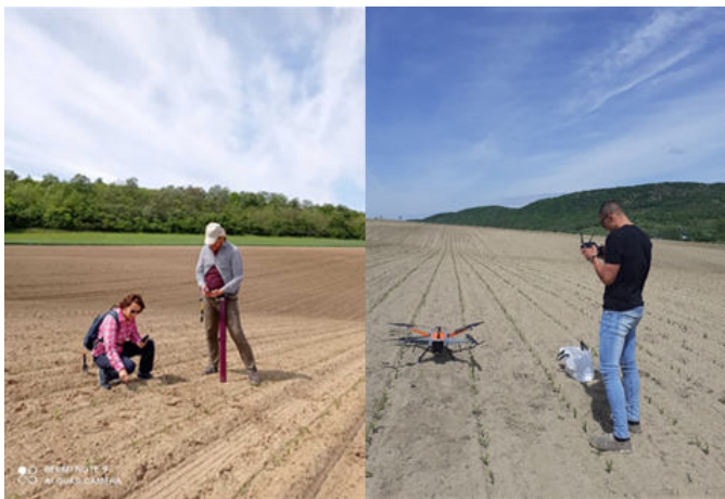
Fig. 5. Field data collection, UAV aerial photography and LIDAR laser scanning of the agricultural field "Csolnok-73"
