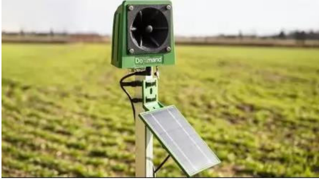
Figure 8 Solar panel powered ultrasonic game alarm [5]
