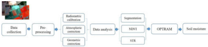
Fig. 8. Satellite data analysis steps for mapping surface soil moisture with OPTRAM algorithm. [18]
