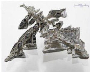
Fig. 7. Surface of bulk tin that to shows typical dendritic crystallization structure obtained at a relatively low cooling rate, [9].
