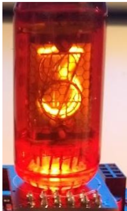
Figure 2: Fog discharge in Nixie tube
