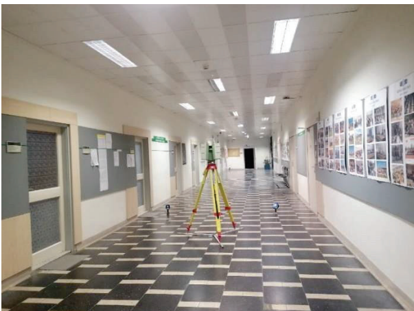
3. Figure - Leica ScanStation C10 laser scanner
