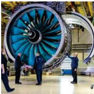
Fig. 1. Roll Royce UltraFan Jet Engine (Source: ROLLS-ROYCE. Digital Twin [online]. [cit. 2025-03-02]. Available at: https://www.rolls-royce.com/innovation/digital/digital-twin.aspx )
