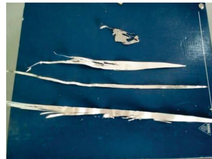
Fig. 3. Prepared metallic glass melt-spun ribbons
