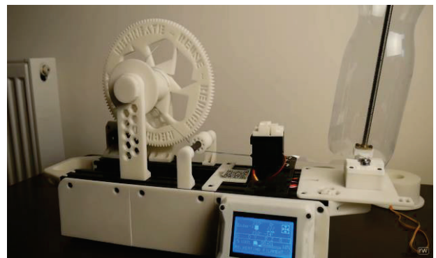
Fig. 6. The filament production process from PET bottle
