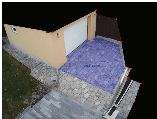
Fig. 5. Example of a motion mask and a zone named “test_zone.” Zone vertices (blue) and motion mask vertices (red) are specified by their (x, y) coordinates. The black area formed by the red vertices represents the motion mask, while the blue area formed by the blue vertices represents the zone. The image coordinate system has its origin at the top-left corner (0, 0) and extends to the bottom-right corner (2560, 1944) .
