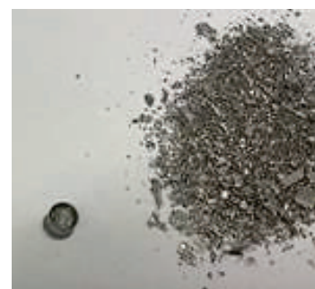
Fig. 4. Fragments of the Al–Sn alloy and pellet produced by pressing
